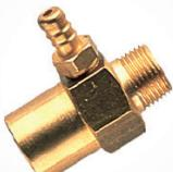
The ejector is simply a “Venturi” which permits sucking up detergent at high pressure. Comet offers two types of ejectors for sucking up detergent which differ in terms of whether or not they feature a sucked-up liquid flow regulator.
