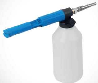
Foam lances are special lances featuring a tank for dispensing sanitizing detergents. Detergent suction is by means of a "Venturi" system at spray gun outlet. This way, the detergent mixed with the water at low pressure generates a thick and effective foam. Comet distributes various kinds of foam lances, from those of the hobby type to professional ones with detergent outlet adjuster, with close focus on the quality of the materials used.
